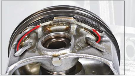
Example of piston damage due to an LSPI event observed during the testing of a competitor's motor oil. The red arrows indicate sections of the ring land that have broken away from the piston.
