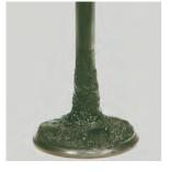
Picture D - Intake valve before P.i. treatment
