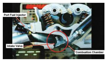
level of oxygen, but not enough fuel, creating a lean misfire that leads to drivability issues such as stumbling, stalling and rough idle. By removing these deposits, all the fuel from the injectors is able to enter the combustion chamber.
