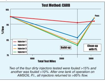
Whether deposits have built up over a relatively low number of miles, as in the test, or they have accumulated over 100,000 miles, P.i. effectively removes them. Because fuel injector deposits and the associated performance issues usually build up slowly over time, motorists often attribute the decreased performance to the increased age of the vehicle. When the deposits are removed in only one tank of gasoline, the performance improvement is immediate and significant.
